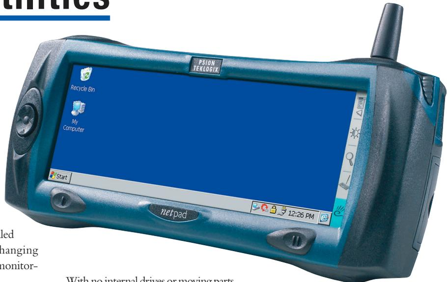
With no internal drives or moving parts, and the ability to withstand a 1.5-meter drop to concrete, the netpad performs in demanding environments, gives more than eight hours of continuous use on one battery charge, and features instant-on capabilities.
